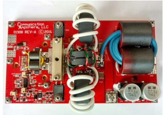
1.8-54MHz, 1000 Watt CW/PEP Class AB Linear Amplifier
